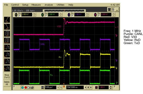
Figure 5. S is Close  $\rightarrow$  V33 Transient at Recessive State (TxD = 1)
