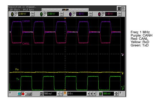
Figure 3. S is Open, V33 is Lost for Transceiver Only, Transmission is Still Possible
