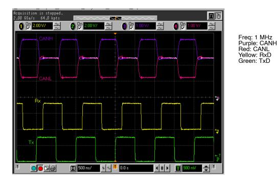
Figure 2. Normal Communication, S Closed V33 Present, Communication via TxD
