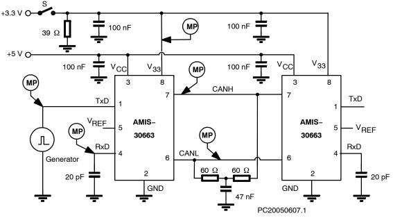
Figure 1. Measurement Set-Up
