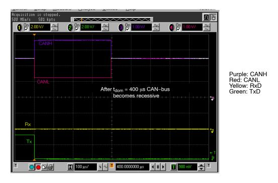
Figure 6. S = Open, V33 is Lost for Both Transceivers as Controller, After the Dominant Time–Out the CAN–Bus Becomes Recessive
